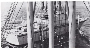
■ Below: deck patrol for Clan Line? This Vosper Thornycroft patrol craft was stowed diagonally across No. 2 hatch of Clan Maclean. It was loaded off Portsmouth May 12 and discharged at Zanzibar June 6—both times by ship's gear. Picture: Capt. M. Brackenridge.
